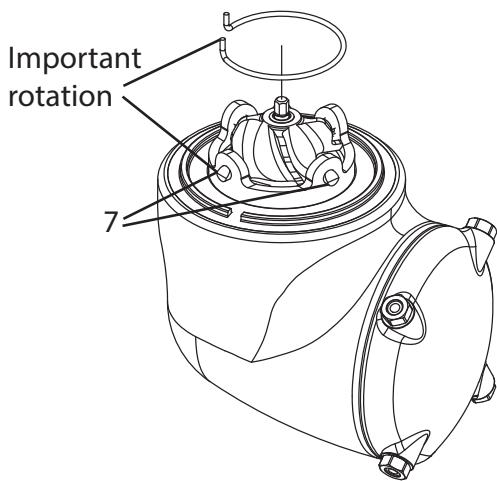
14. Also mount the pins on the locking ring (pos. 6) facing upwards.
