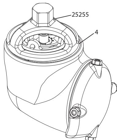
6. Remove ball race and stator.
