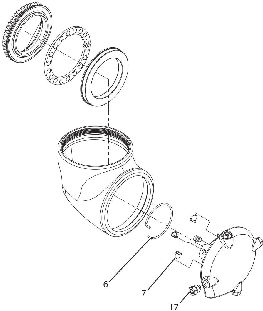
12. Remove the vertical gear and gear shaft in the same way.
