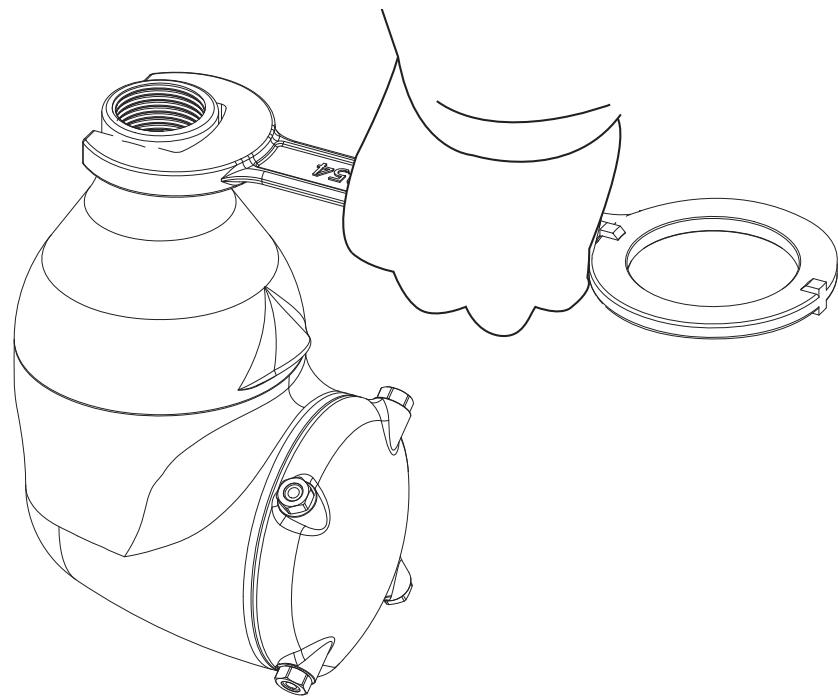
When threading the inlet connection of the tank cleaning machine to the cleaning media connection, Scanjet recommends that Food Grade Teflon tape or any other appropriate food grade anti-seizing compound is used to avoid metal galling (Galling means that threads clamp together and cannot easily loosen).
