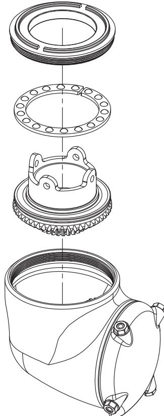
7. Undo the three bolts (pos. 12) holding the gearbox in position, and then remove the gearbox. Be careful not to damage the gears!
